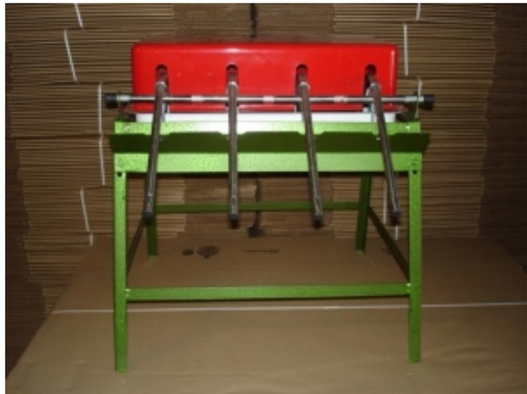
Several styles of gravity type bottle fillers are available. These fillers have a small tank to hold the wine and two or more siphon tubes to transfer the wine into the bottles. A float-valve mechanism is used to keep the tank full. Operation of small multi-spout, gravity type fillers is simple. An empty wine bottle is placed on a spout. The machine fills the bottle to a preset level and automatically stops. Two, three, four
