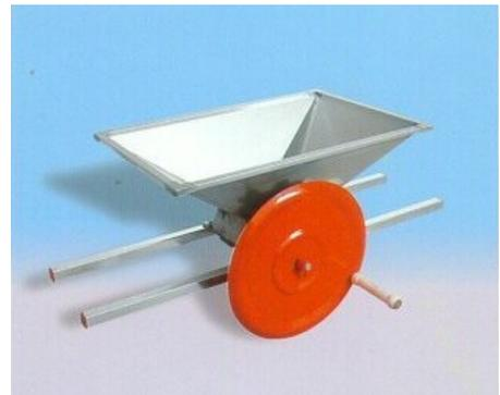
crusher designs are easy to crank and some are not. Operation of these little crushers is quite simple. The crusher is placed on top of a suitable container. The hopper is filled with fruit, and the crank is turned. Clusters of grapes pass through the rollers and the crushed fruit and stems drop into the container. Having some way of clamping the crusher on the container is very desirable. If the crusher slides or moves around, it will be more difficult to crank.
