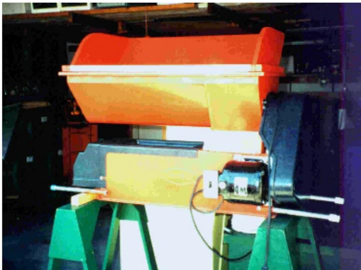
Power crushers have capacities ranging from about 1 ton to more than 50 tons per hour. Even the smallest machines crush and destem large quantities of fruit in a short time. One person is busy keeping the hopper full of grapes.
