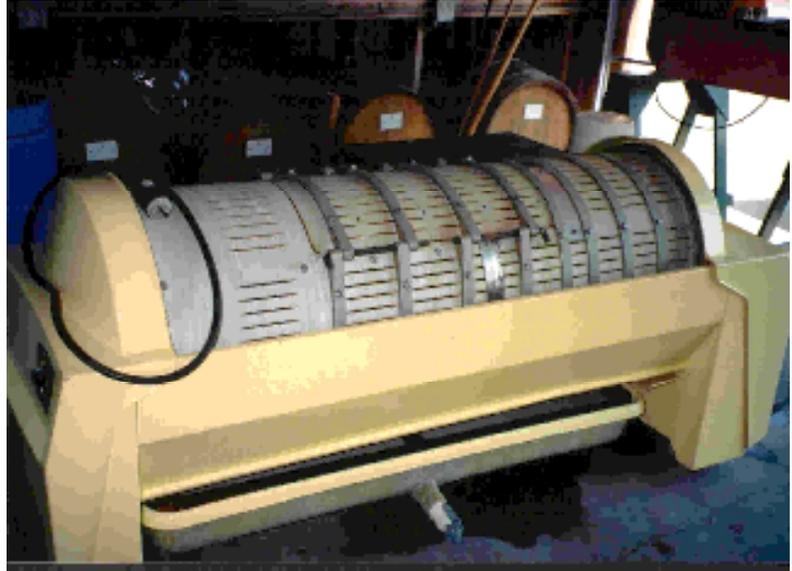
Computers control Modern commercial winepresses, and they can be programmed to execute very complicated press schedules automatically. Modern presses use an inflatable bag, tube or membrane. After the press is loaded, the membrane is inflated and gently squeezes the grapes against the basket to extract the juice.
